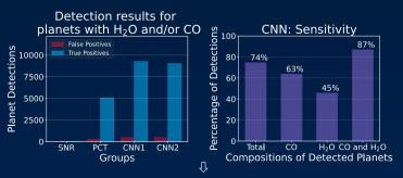
By construction, our CNNs use molecular templates as filters (c.f. paper). Thus, we tested the possibility to include templates from two molecules simultaneously, to detect planets without making assumptions on the composition. We find that by doing so, the CNNs effectively combines information of each template to detect planets containing both molecules, but can also detect planets with either one of the molecules.
