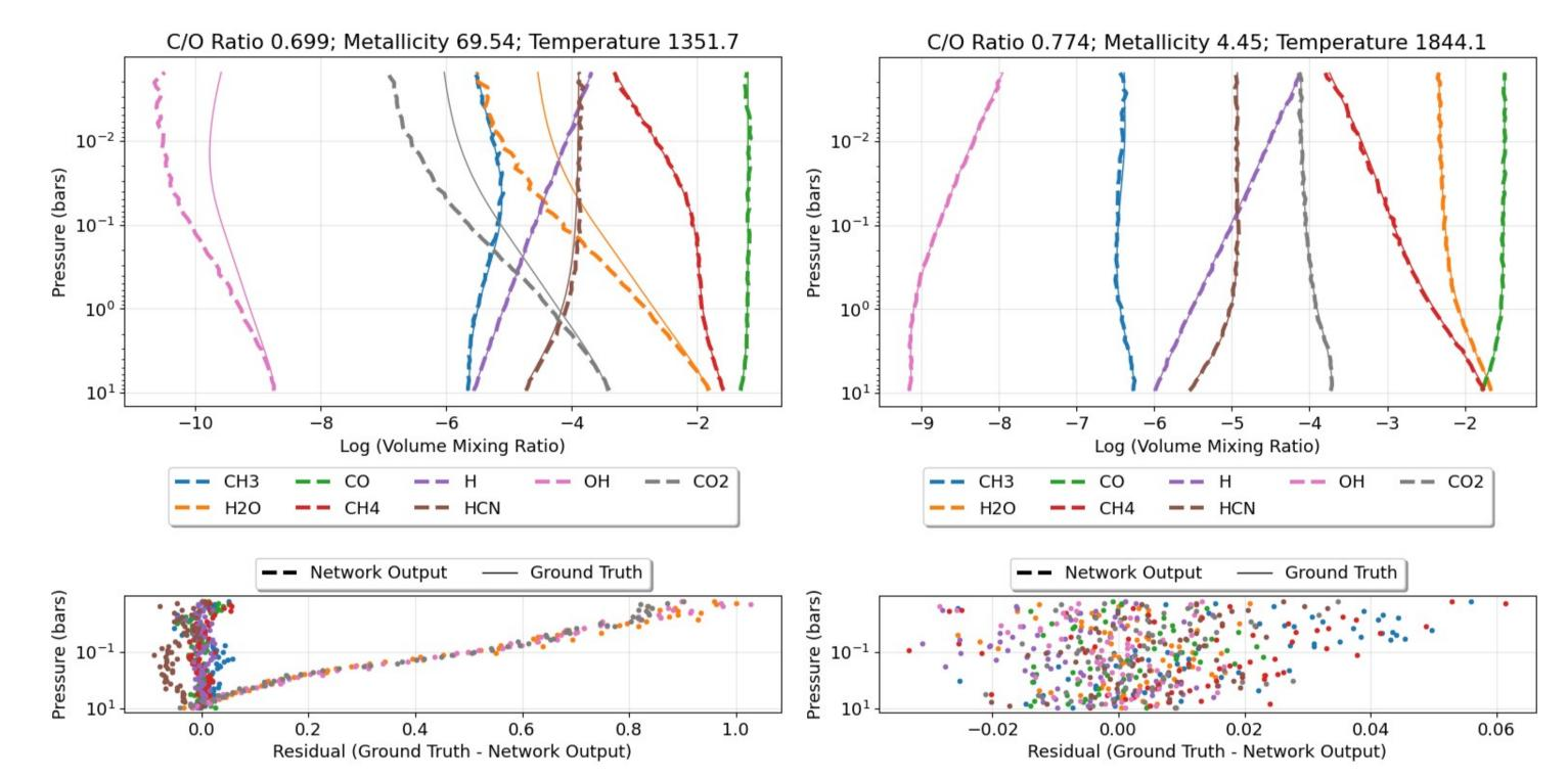
Figure 3: Log volume mixing ratios against pressure, with the C/O ratio, Metallicity, and Temperature noted above the plot. The left plot shows the worst prediction by the network, while the right plot shows the average prediction by Chexanet. Dashed lines represent neural network predictions, while solid lines indicate ground truth data. Below the main plots are residual plots between ground truth and network output, emphasising the variability in performance for different molecules.
